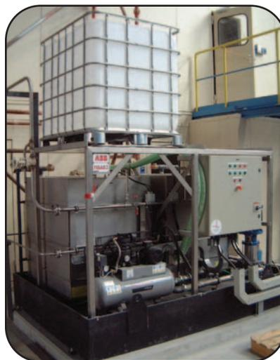
*Turbotect's new 2020 cleaning solution for off- and on-line compressor washing is water based and has been specially developed to address the type of fouling found in today's gas turbines.*
